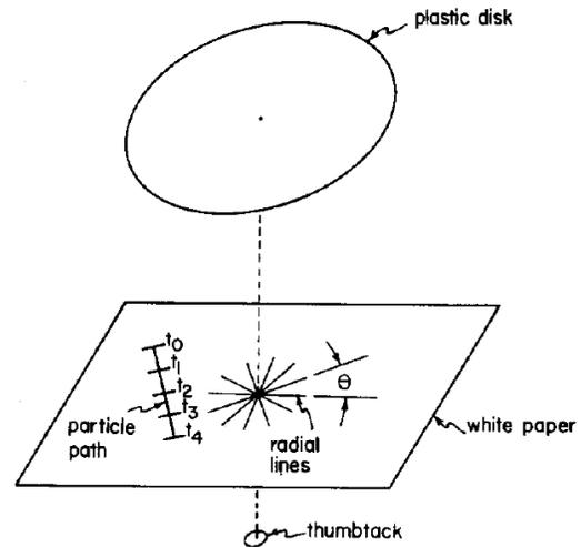
Fig. 1. Exploded view of Coriolis machine.
